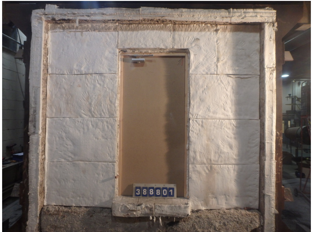
The exposed face of the Doorset prior to the start of the test
