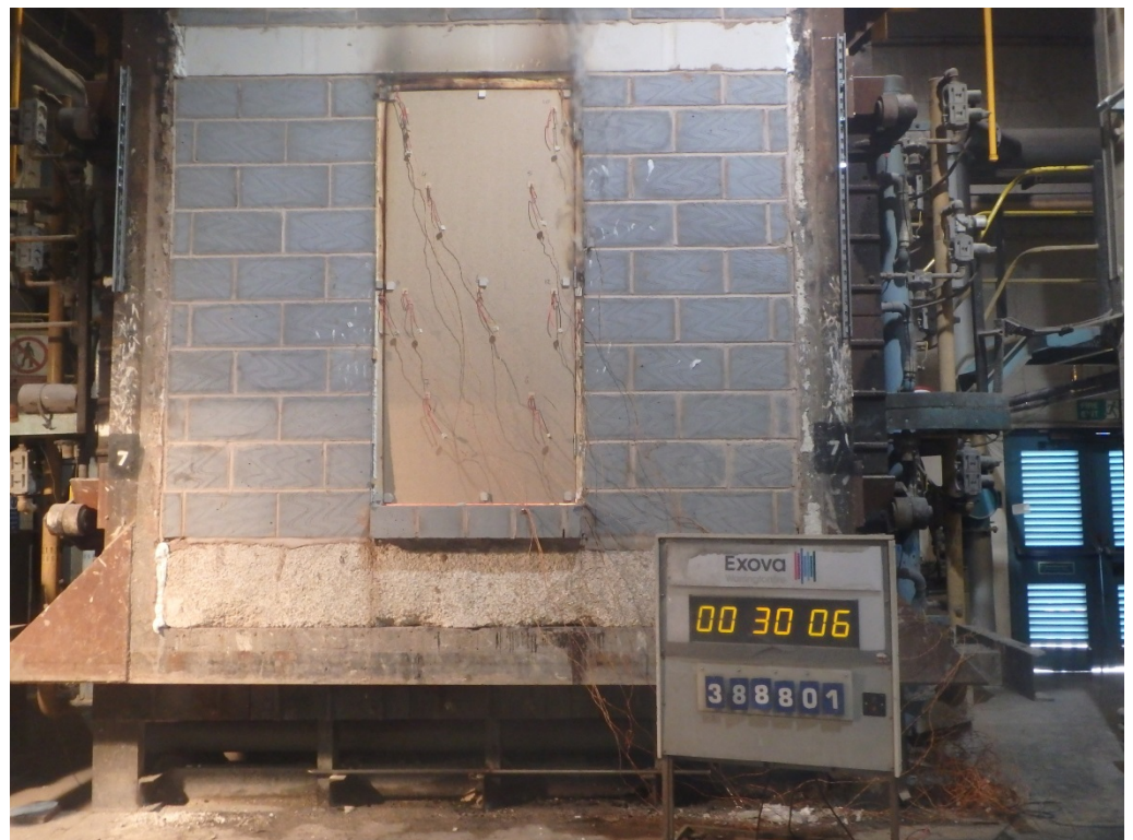
The unexposed face of the Doorset after a test duration of 30 minutes
